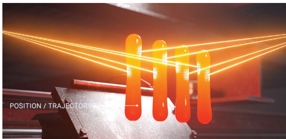
The high speed matrix cameras can still monitor partially obscured gobs.
